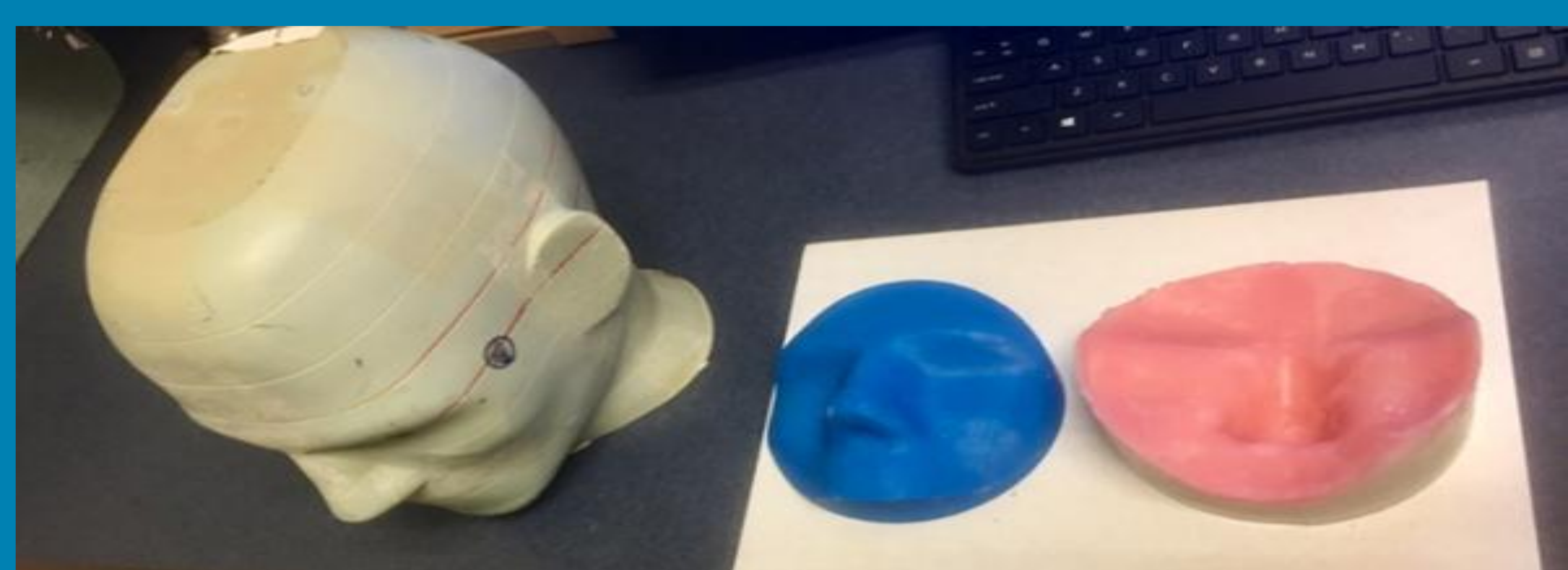
Figure 3: Construction of the wax bolus with 3D printer.
